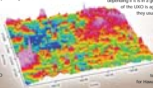
Side View of Detected Anomalies: This particular 100m grid, in a heavily-used target area near the center of Kahoolawe Island, produced 733 anomalies which were mostly UXO fragments or remnants.
